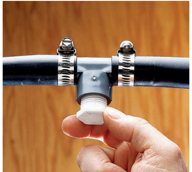
Connect lengths of PE pipe with a barbed PVC fitting. Secure the connection with stainless steel hose clamps.
