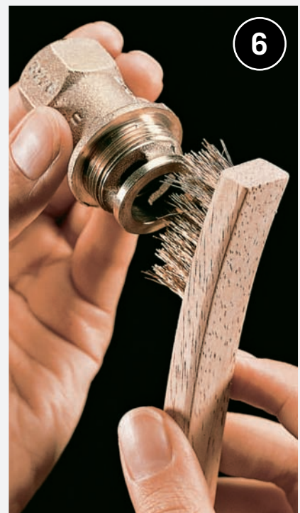
Clean sediment and lime buildup from nut, using a small wire brush dipped in vinegar. Coat all parts with faucet grease and reassemble diverter valve.
