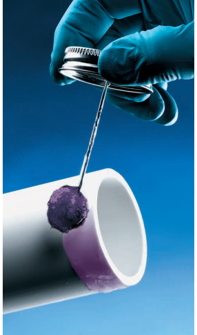
Solvent welding is a chemical bonding process used to permanently join PVC pipes and fittings.
