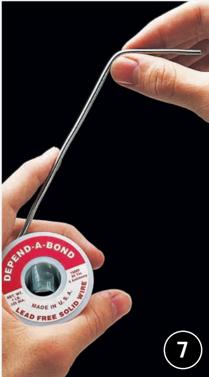
7 Prepare the wire solder by unwinding 8" to 10" of wire from spool. Bend the first 2" of the wire to a 90° angle.
