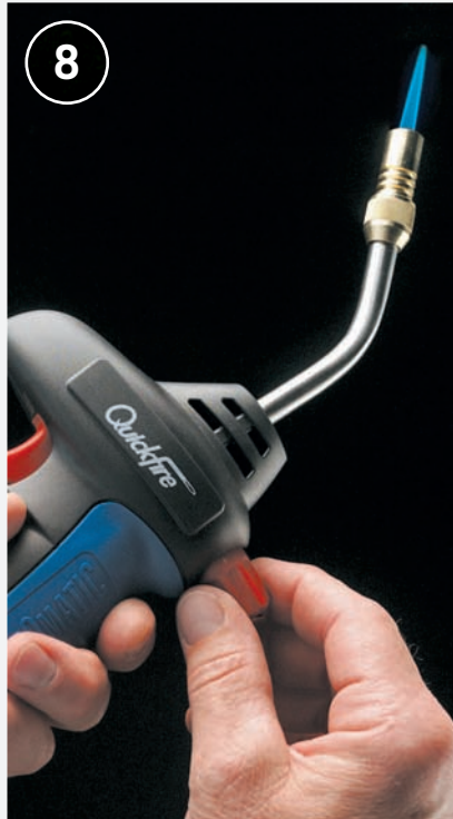
8 Open the gas valve and trigger the spark lighter to ignite the torch. Adjust the torch valve until the inner portion of the flame is 1" to 2" long.
