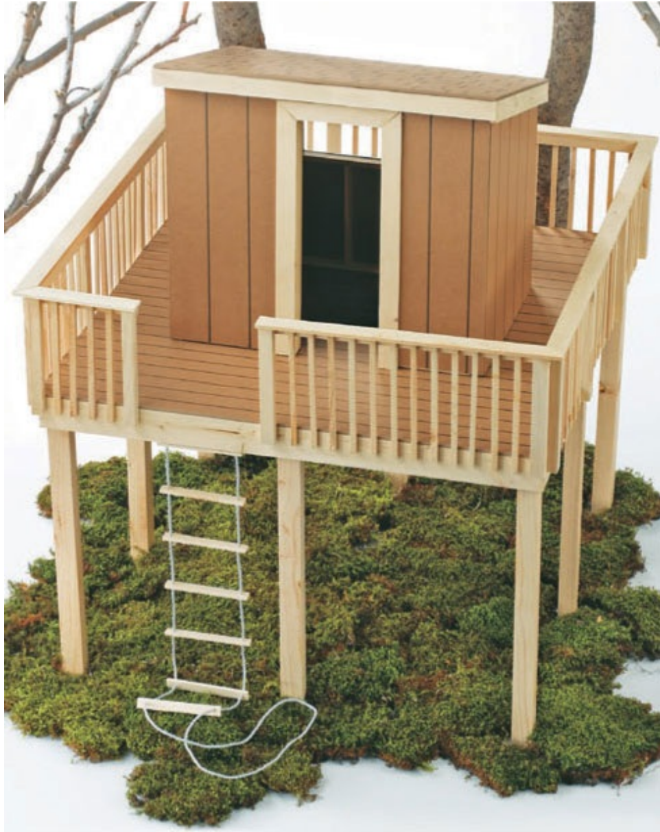
Centering a small house on a platform makes an instant wraparound deck.
