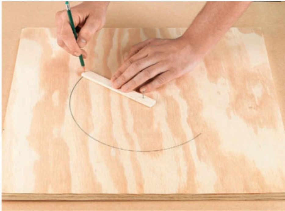
Mark the circular cutting line of the disc using a homemade compass.
