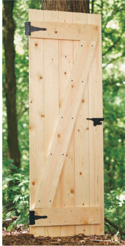
A plain batten door made from 1 x 6 pine has a certain rustic charm. A single Z-brace stiffens the door, but adding a middle rail and second Z-brace prevents warping.
