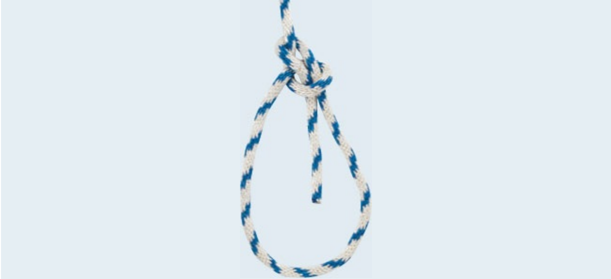
Step 3: Tighten the knot by holding the working end in place while pulling up on the standing portion.
