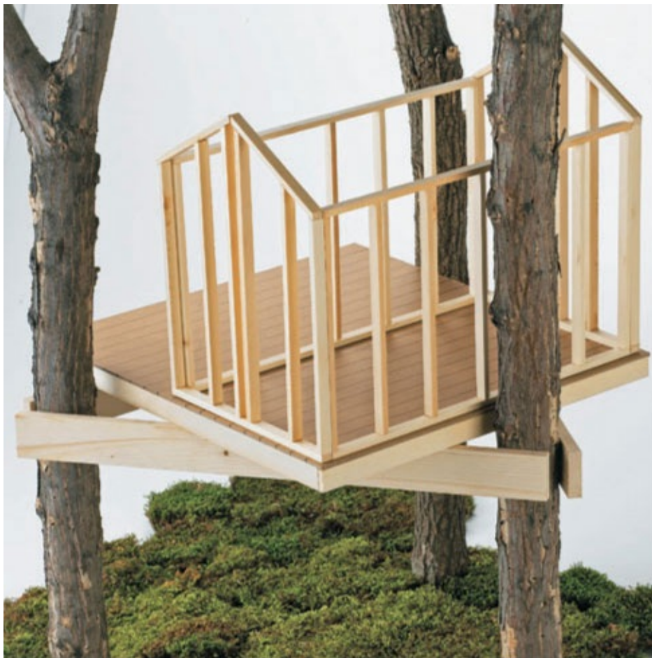
Gable end wall layout with 30° roof pitch.
