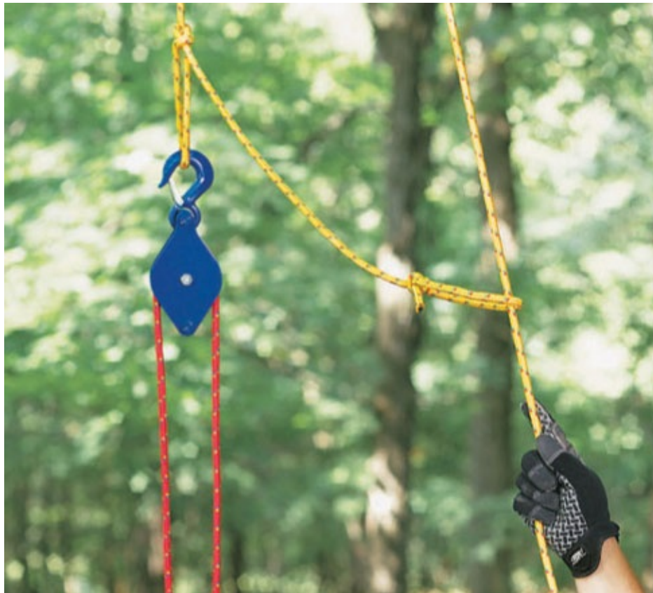
One rope raises and affixes the pulley to the tree; a second rope operates the pulley.
