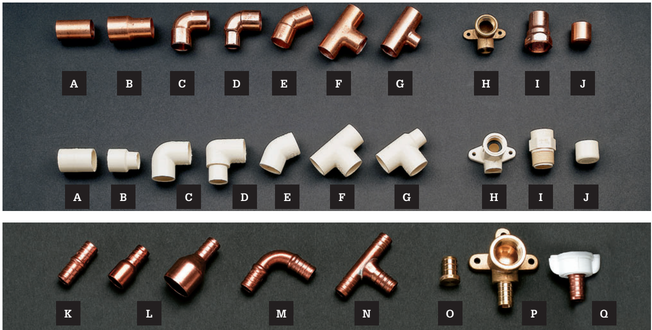
Water supply fittings are available for copper (top), CPVC plastic (center), and PEX (bottom). Fittings for CPVC and copper are available in many shapes, including: unions (A), reducers (B), 90° elbows (C), reducing elbows (D), 45° elbows (E), T-fittings (F), reducing T-fittings (G), drop-ear elbows (H), threaded adapters (I), and caps (J). Common PEX fittings (bottom) include unions (K), PEX-to-copper unions (L), 90° elbows (M), T-fittings (N), plugs (O), drop-ear elbows (P), and threaded adapters (Q).
