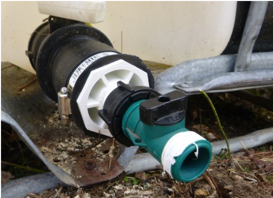
A rubber connector and PVC pieces make it simple to manage water coming out of an IBC tank.
