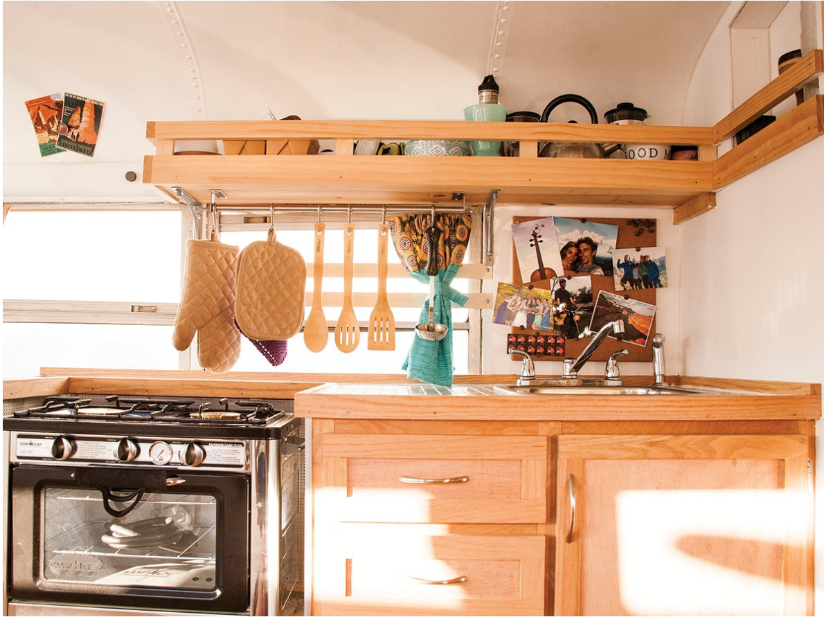
The compact kitchen includes a small sink and a Camp Chef propane camping oven, surrounded by decorative metal sheeting. Pots, pans, and dishes are stored in oak-faced drawers, and a rack for hanging utensils allows for easy access. The glass-tile countertop has a small lip around it to stop things from slipping off.
