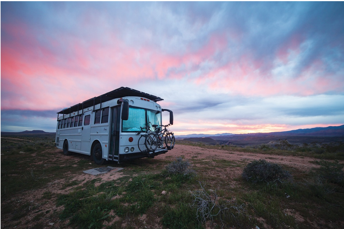
The bus's steel roof rack was custom made by a metal fabrication company. The rack constituted one of the bigger costs of the bus at $4,500, but it allows the couple to haul hefty items. Rooftop solar panels are mounted on hinges at the front of the rack and the tilt of the panels can be
