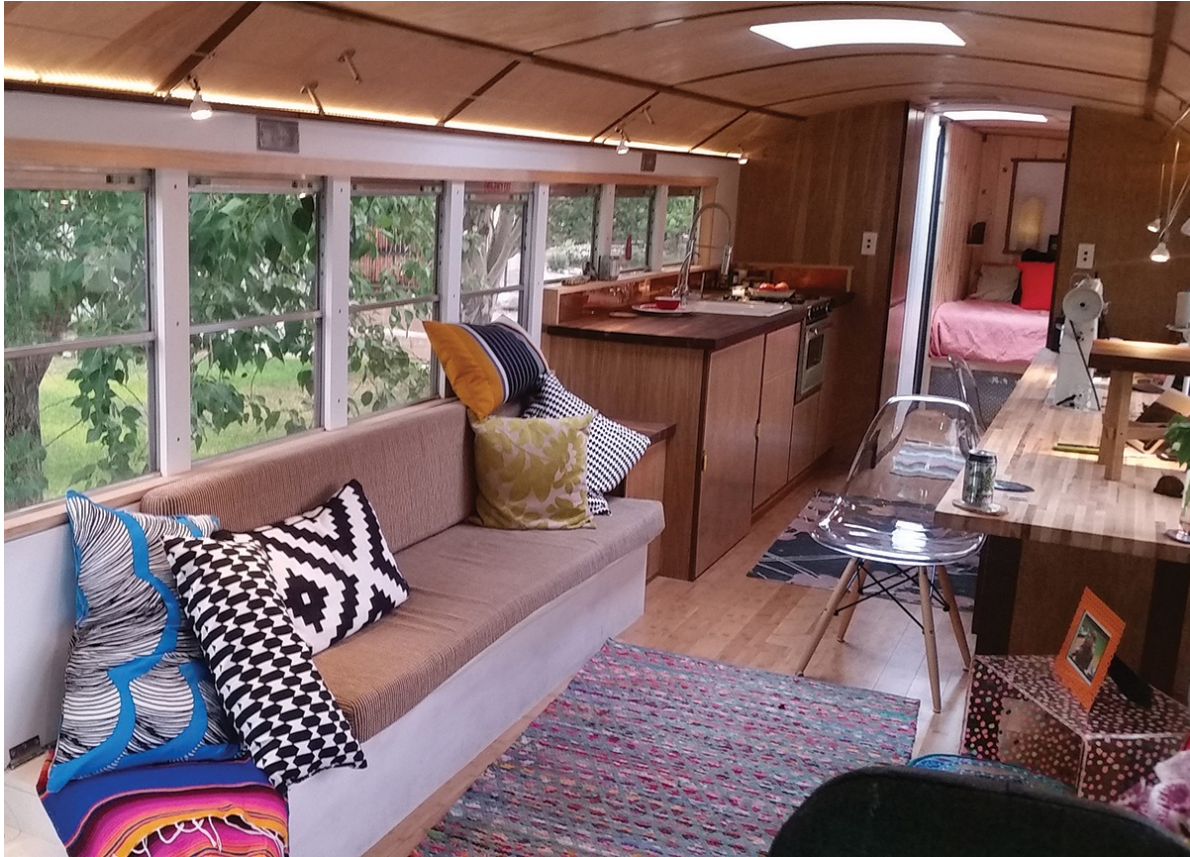
This is Lucy, a 1995 AmTran Genesis school bus conversion done by Art Builders Guild and commissioned by a hat maker. It's her off-grid studio, home, and mobile store. Interesting features include custom oak and walnut cabinetry with a recycled copper backsplash and a chest freezer that has been converted into an extremely efficient refrigerator that uses only one-tenth of the electricity of a regular refrigerator. It is placed on a custom steel rack that can roll in and out of the kitchen counter.
