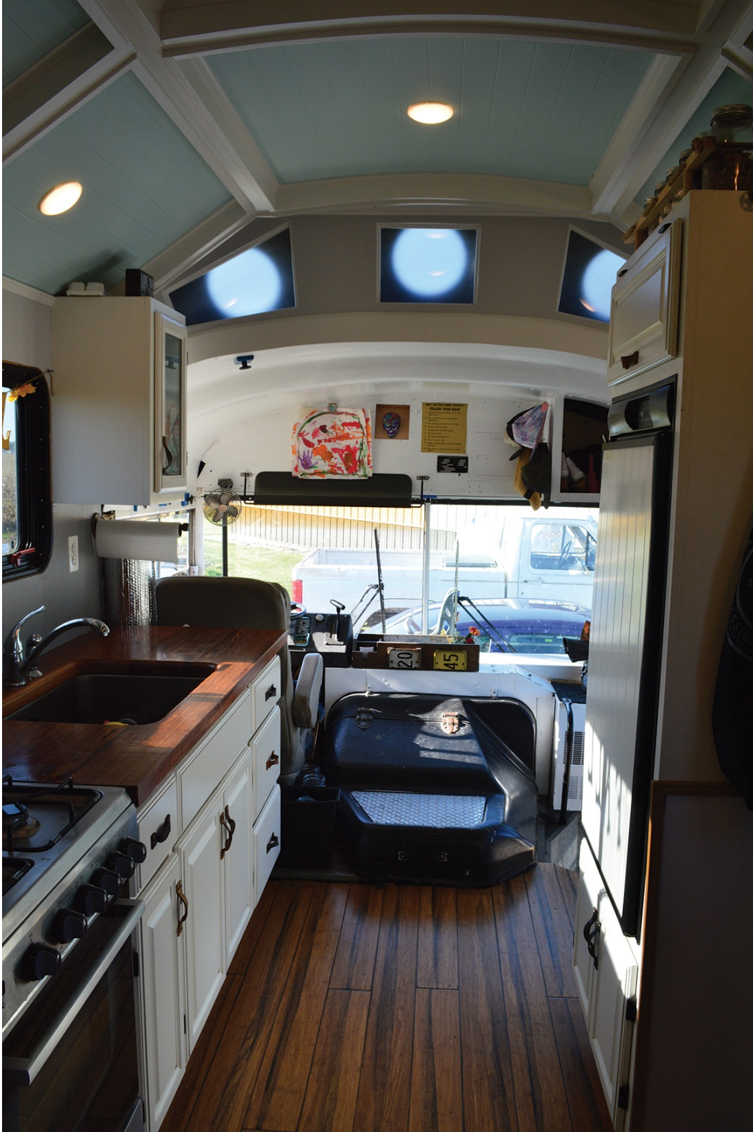
The couple raised the roof almost 2 feet on their renovated 240-square-foot home, adding a significant amount of headroom to the interior space. This also permitted them to add a lofted
