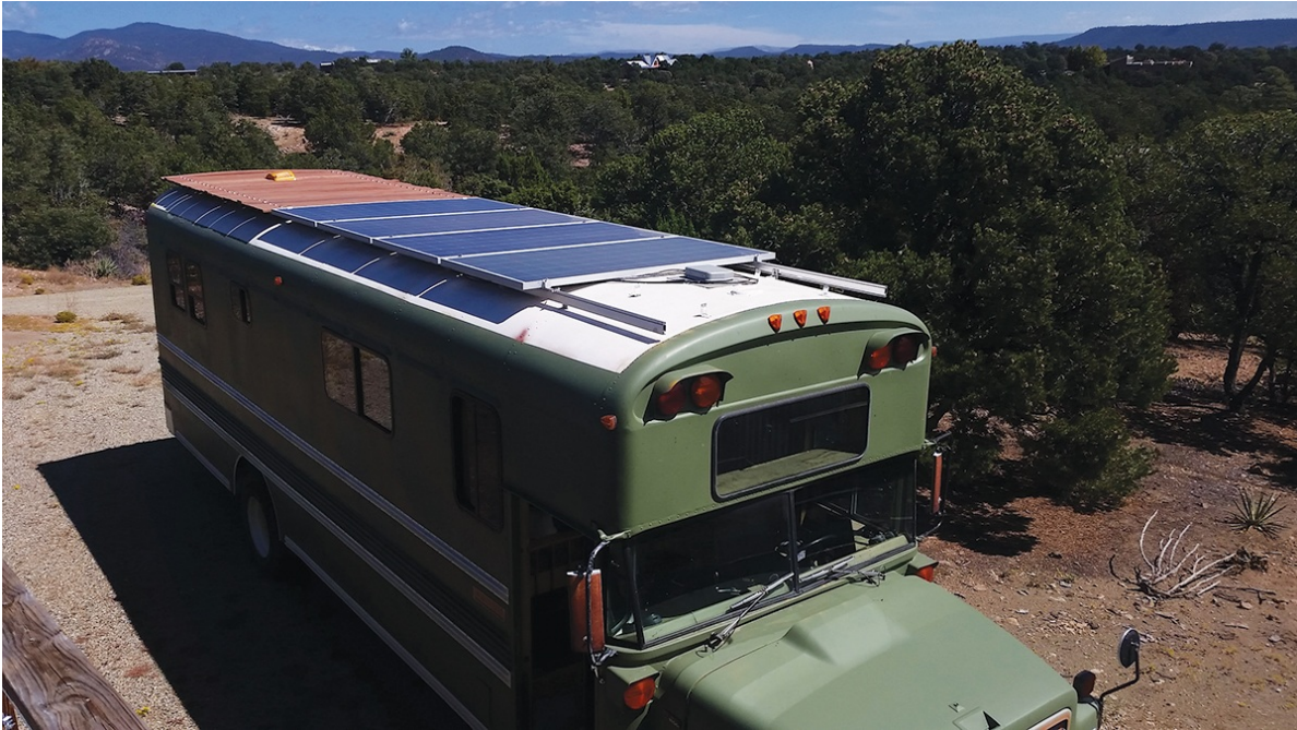
The Queen is equipped with a 1,875-watt solar panel array—more than enough power for a vehicle of this size, and sufficient to run lights, gadgets, the water heater, and the air-conditioning during the summer.
