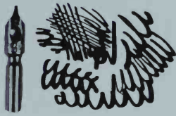
Wm Mitchell 0851, a stiff, flat-pointed lettering pen producing a heavy line in one direction and a finer line in the other.
