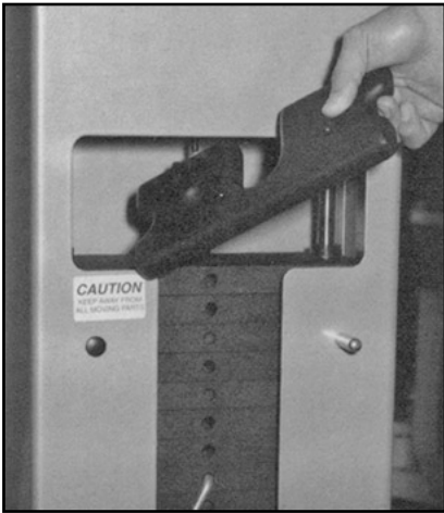
A weight designed to fit on top of a selectorized weight stack.
