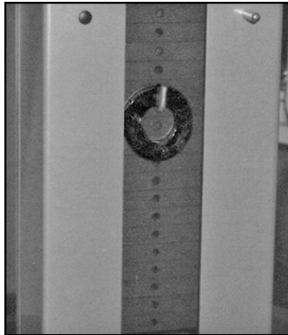
A little plate “pinned” to the stack, for a small increase in weight—a microload.
