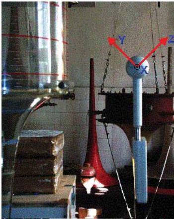
Figure 5: Position of the ESM-100 probe sideways, with indication of the coordinate system
