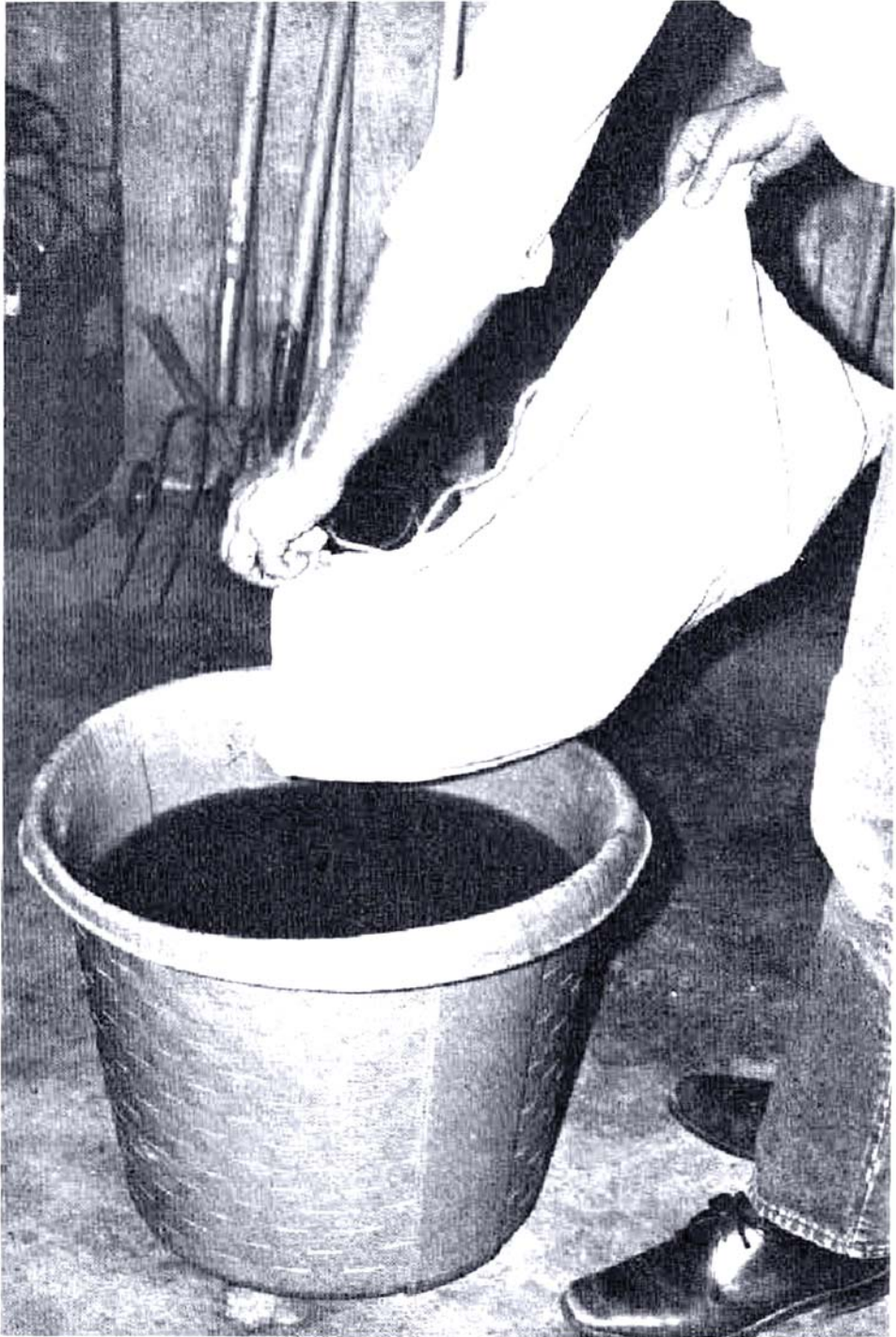
Hair must be removed from skins used to make leather. Lime is added to clean water, and the skins soaked again until the hair comes loose. Hair is then scraped off before continuing the leather-making process.
