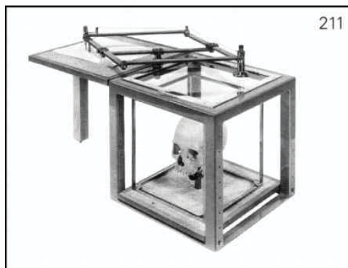
Quadratic dioptograph (Martin). Weight: 10.00 kg.
