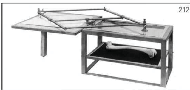
Rectangular dioptograph. Weight: 15.500 kg.
