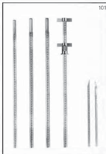
Anthropometer. Scale: 0-2100mm (0-960mm) for determination of all vertical lengths on the body. Weight: 1.450 kg.
