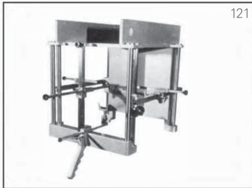
Anthropostereometer for measurement of the head and skull. Weight: 11.08 kg.
