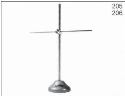
Left: Stylus for guiding horizontal lines. Height: 450-mm. Weight: 1.300 kg. Right: Tubular craniophor (Martin) with a device for measuring the height of the ears (Black). Weight: 2.100 kg.
