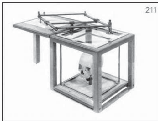
Quadratic dioptograph (Martin). Weight: 10.00 kg.
