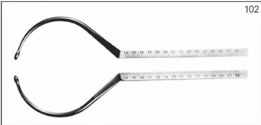
Curved gaging arcs for anthropometrics; for example, for measurement of the sagittal diameter the chest. Weight: 0.170 kg.
