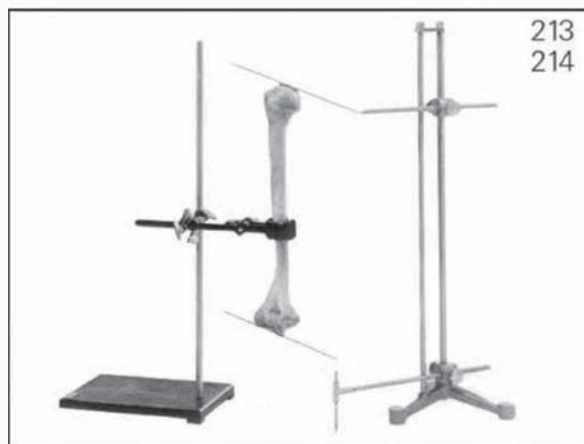
Parallelogram (Martin) for measurement of the angle of the axes of the joints. Weight: 1.600 kg. Weight of bone holder: 2.400 kg.
