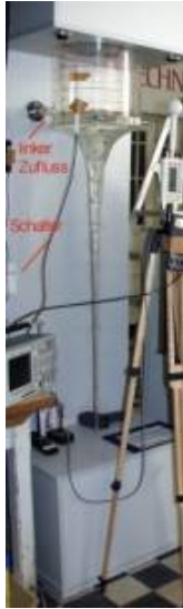
Figure 1: Hyperbolic funnel, experimental set-up
