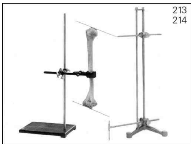
Parallelogram (Martin) for measurement of the angle of the axes of the joints. Weight: 1.600 kg. Weight of bone holder: 2.400 kg.
