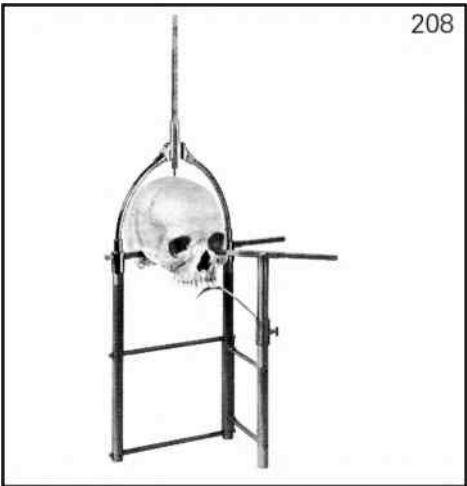
Craniophor (Mollinson) specifically for mounting the skull on the plane of the ears-eyes. Weight: 1.870 kg.
