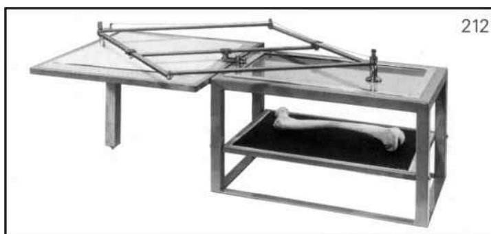
Rectangular dioptograph. Weight: 15.500 kg.
