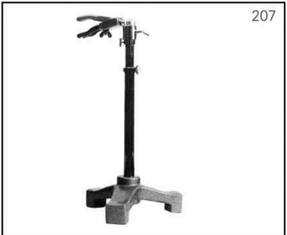
Left: Stylus for guiding horizontal lines. Height: 450-mm. Weight: 1.300 kg. Right: Tubular craniophor (Martin) with a device for measuring the height of the ears (Black). Weight: 2.100 kg.
