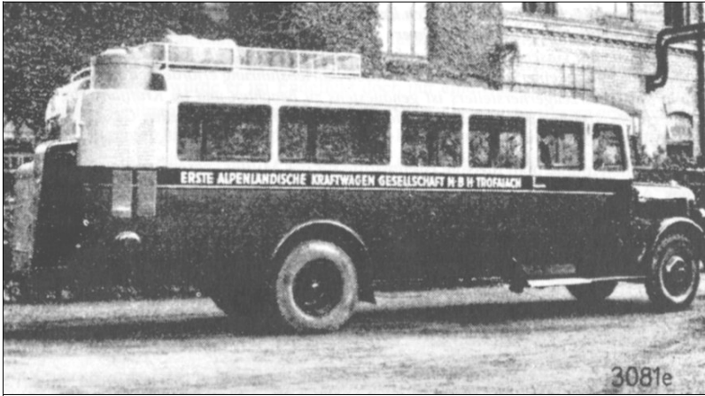
Illustration 1: A typical gaswagen which had originally been a conventional bus but which was subsequently retro-fitted with a gas-generator and a Saurer engine. 81
