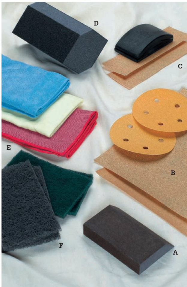
Smooth, even surfaces are easy to achieve with tools such as these: sanding sponges (A), sandpaper (B), sanding block (C), a drywall-corner sanding sponge (D), microfiber tack cloth (E), and synthetic steel wool (F).
