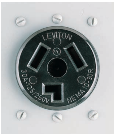
30 amps, 120/240 volts. This receptacle is used for clothes dryers. It provides high-voltage current for heating coils and 120-volt current to run lights and timers.
