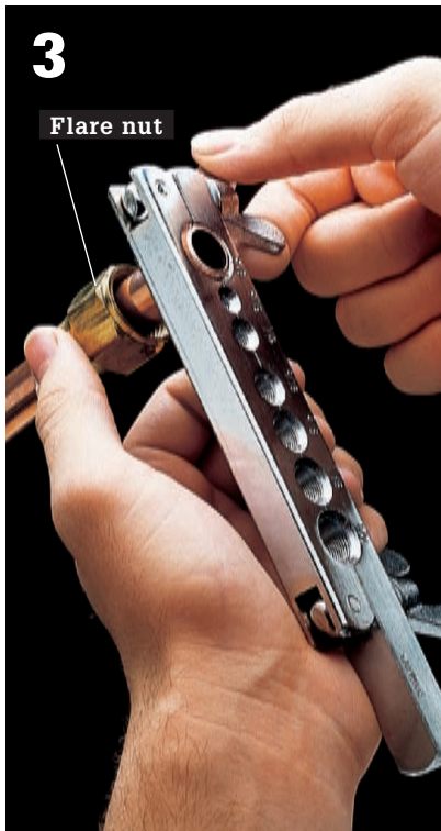
3 Clamp pipe inside flaring tool base. End of pipe must be flush with flat surface of base.
