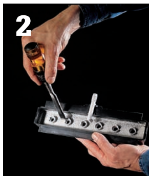
2 Use a chisel to scrape mineral deposits from the V-notches.
