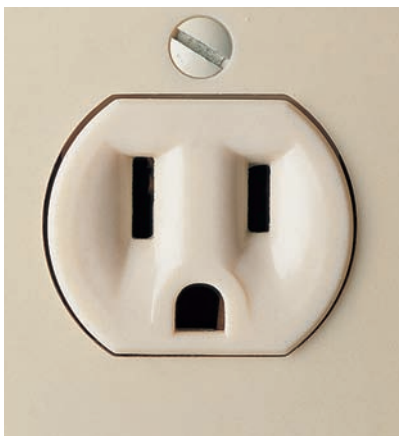
15 amps, 120 volts. Three-slot grounded receptacle has two different size slots and a U-shaped hole for grounding. It is required in all new wiring installations.
