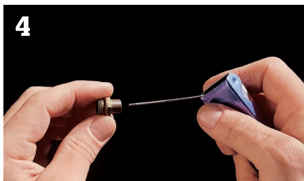
4 Clean each spud orifice carefully with a pilot jet tool, taking care not to scratch or enlarge the orifice.
