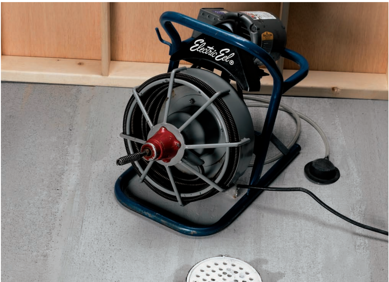
When the going gets tough , the tough rent power tools. The medium duty auger shown here is perfect for augering the 2-inch-diameter floor drainlines and branch drainlines.
