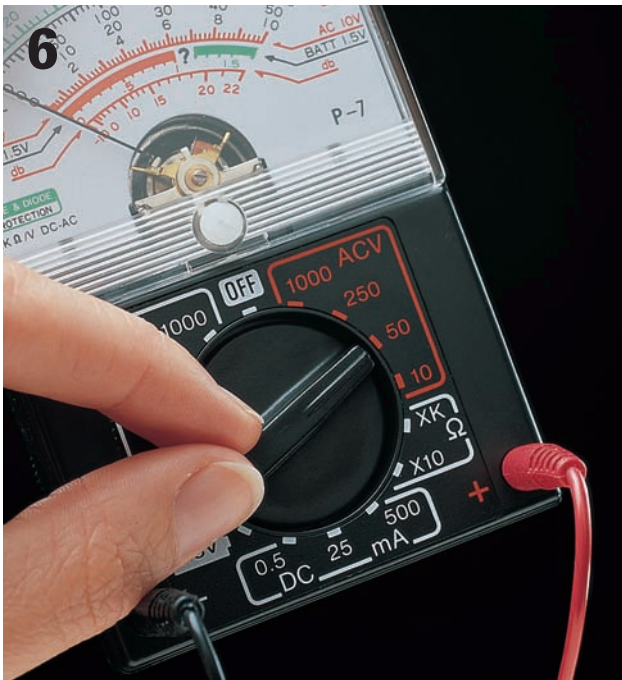
6 Set a multimeter to the 50-volt (AC) range. Turn on power to the heating/air-conditioning system at the main service panel.
