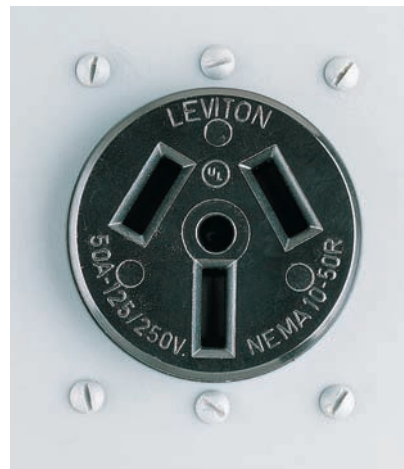
50 amps, 120/240 volts. This receptacle is used for ranges. The high-voltage current powers heating coils, and the 120-volt current runs clocks and lights.
