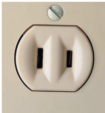
15 amps, 120 volts. Polarized two-slot receptacle is common in homes built before 1960. Slots are different sizes to accept polarized plugs.
