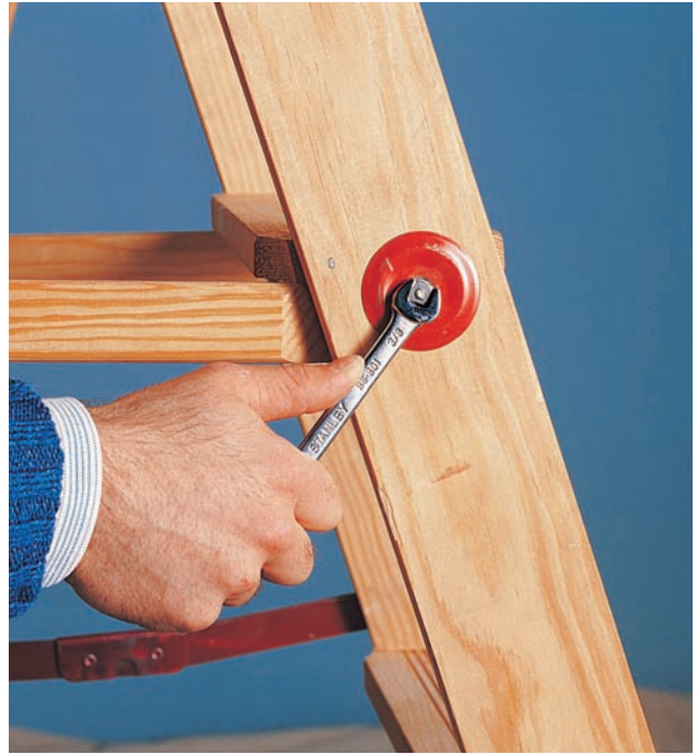
Keep steps tight by periodically checking them and tightening the braces when they need it.
