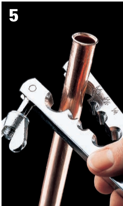
5 Remove yoke and remove pipe from base. Repeat flaring for other pipe.
