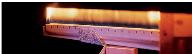
1 Compare your burner flame with the two above. Yours should be blue-green, with streaks of yellow (top).
