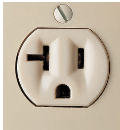
20 amps, 120 volts. This three-slot grounded receptacle features a special T-shaped slot. It is installed for use with large appliances or portable tools that require 20 amps of current.
