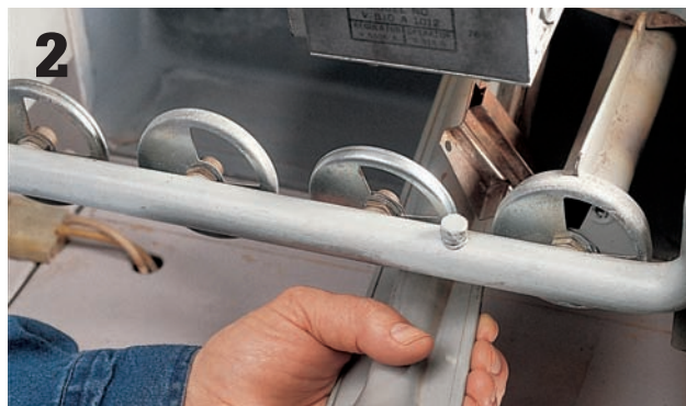
2 If a burner is difficult to remove, twist it carefully from side to side while lifting and pulling.
