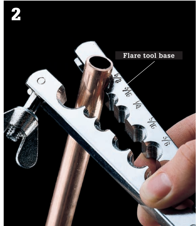
Select hole in flaring tool base that matches outside diameter of pipe. Open base, and place end of pipe inside hole.
