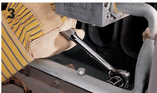
3 To avoid bending or damaging the spud threads, hold the manifold steady with one hand as you remove each spud.
