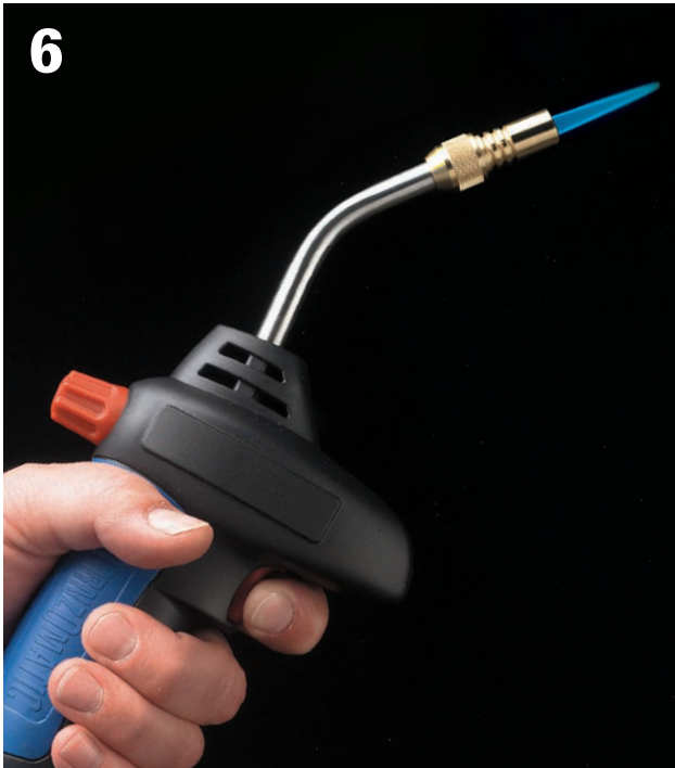
6 Open the gas valve and trigger the spark lighter to ignite the torch.
