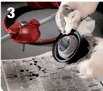
3 Wipe the edge of the cartridge, first with a solvent-dipped rag and then with a dry rag.
