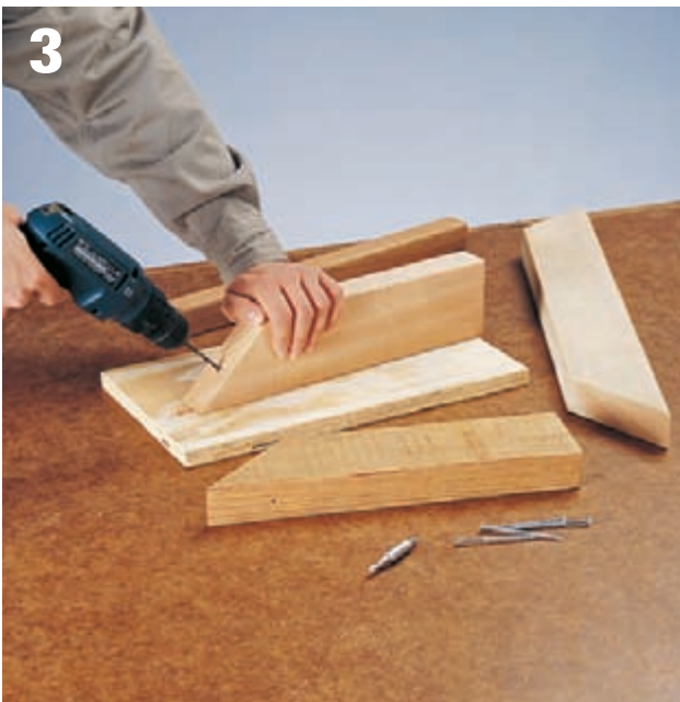
3 Before attaching the cap ends, drill pilot holes through the mitered ends of the cap-front ends.
