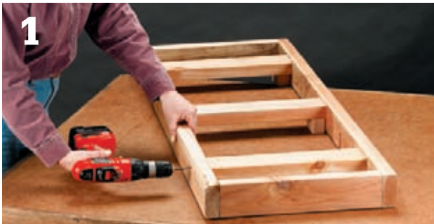
1 Assemble the frame. Use 1\frac{1}{2} " blocks to support the stretchers. Drill pilot holes and fasten the stretchers to the sides with 3" deck screws.
