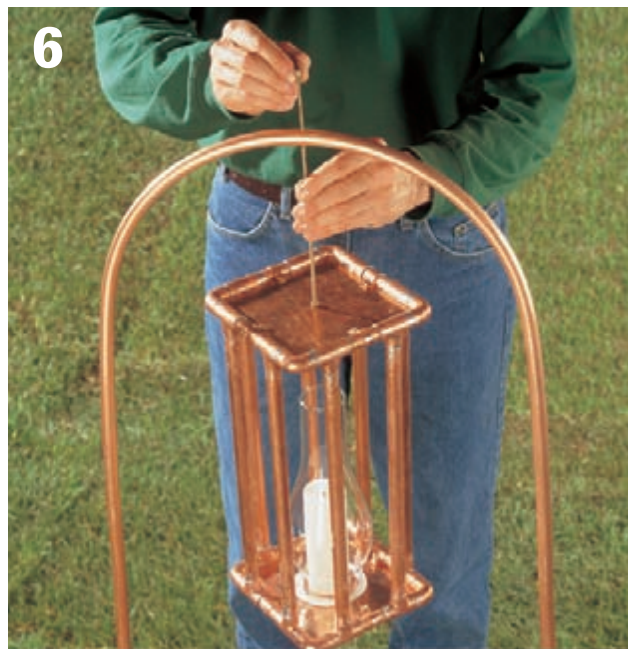
6 Add a nut to the top of the hanging rod; slide it through the hole in the supporting arch. Secure the rod with an acorn nut.
