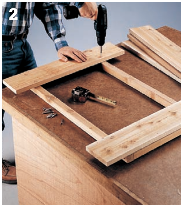
Attach a slat at each end of the panel frame so the outer edges of the slats are flush with the outer edges of the frame.
