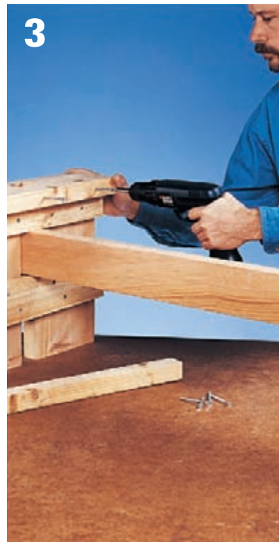
3 Attach the outer brace for the seat slats directly to the inside faces of the cleats.
