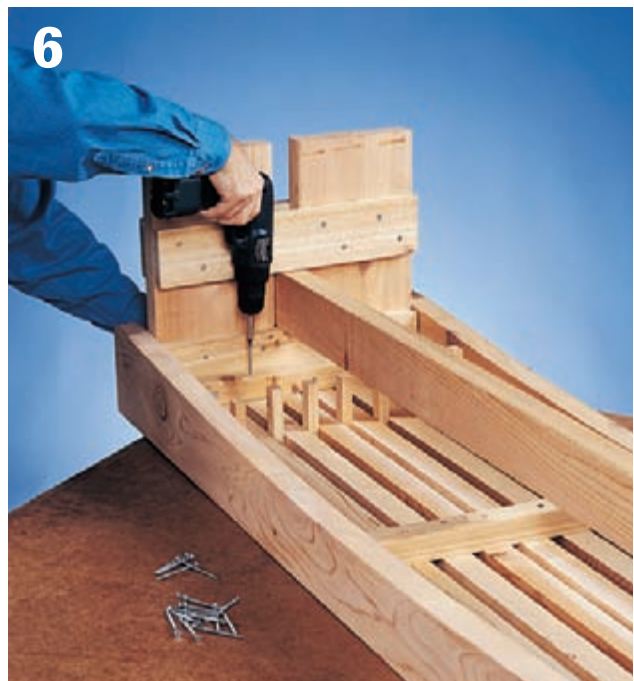
6 Attach the seat slats with glue and 2½" deck screws. Insert ½"-thick spacers to set gaps between the slats.
