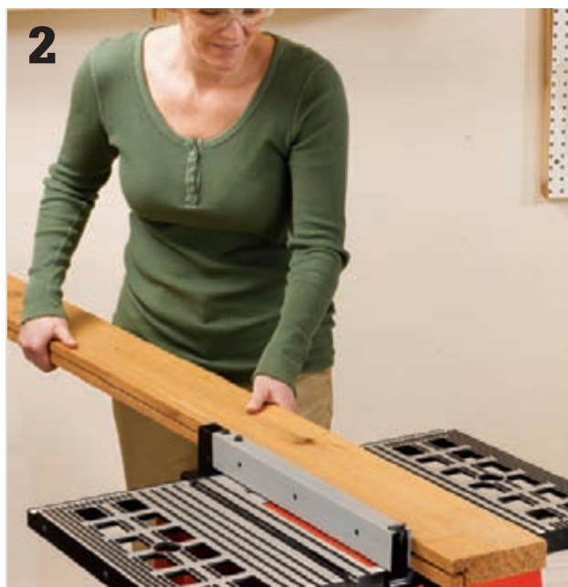
Cut panel rabbets. Make the ¾ × ¾" rabbet cuts in the rail stock using a table saw or router. The rabbets will accept the plywood side panels.
