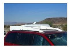
If you look close, you can see that the uprights are held onto the rails with square "U"-bolts. I bought extra cross-straps for the u-bolts so they would take more tension. I also put both the nut that came with the u-bolts AND a nylon-insert, "lock" or "stop" nut. I use "stop" nuts on everything.
