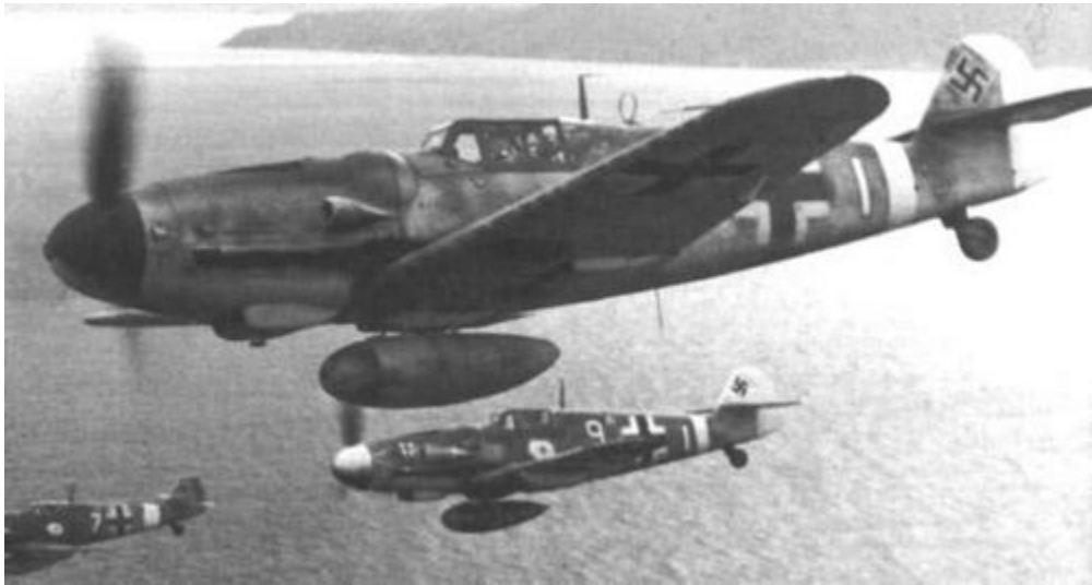
Messerschmitt 109: two guns, two machine guns, 1700 horsepower; 600 kilometres per hour. Together with the Focke Wulff 190 in 1942, it retained air dominance in Russia.
