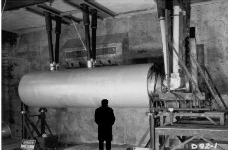
The Castle Bravo Dry-Fueled Deliverable “Shrimp” Device, with a Human Silhouette Superimposed to show approximate size. Compare with the much larger “Mike” device on page 3.
