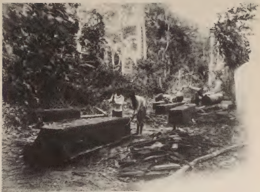
SHAPING TIMBER BY HAND.
