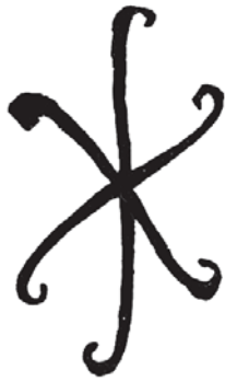
The "German man" as masonry anchor
