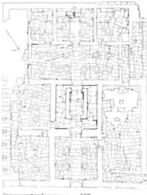
Fig. 4. Survey of the southern part of the covered temple showing the irregularity of the pavement.
