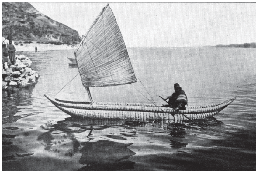
Fig. 6 Indian fisherman in his balsaca made of rush wickerwork with a rush sail on Lake Titicaca. Phot. Professor Arthur Posnansky in La Paz.
