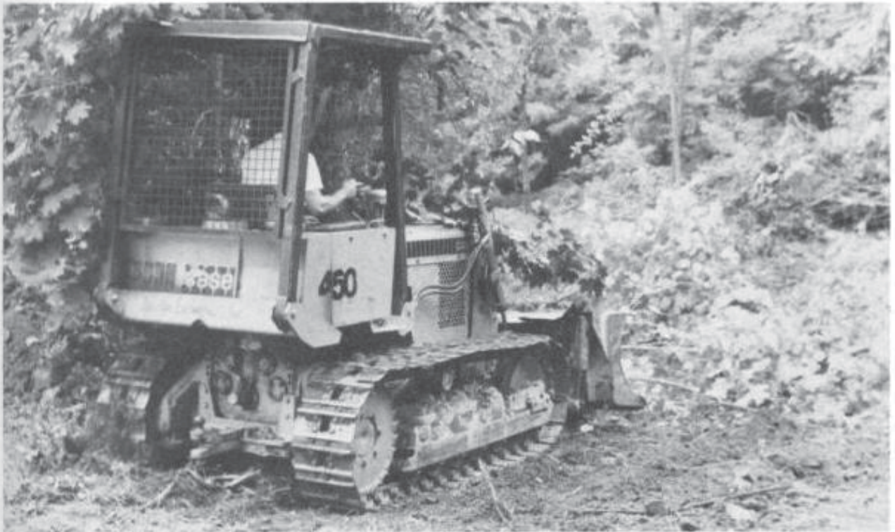
Fig. 4-4. A 450 Case bulldozer is not too small and it's not too large.
