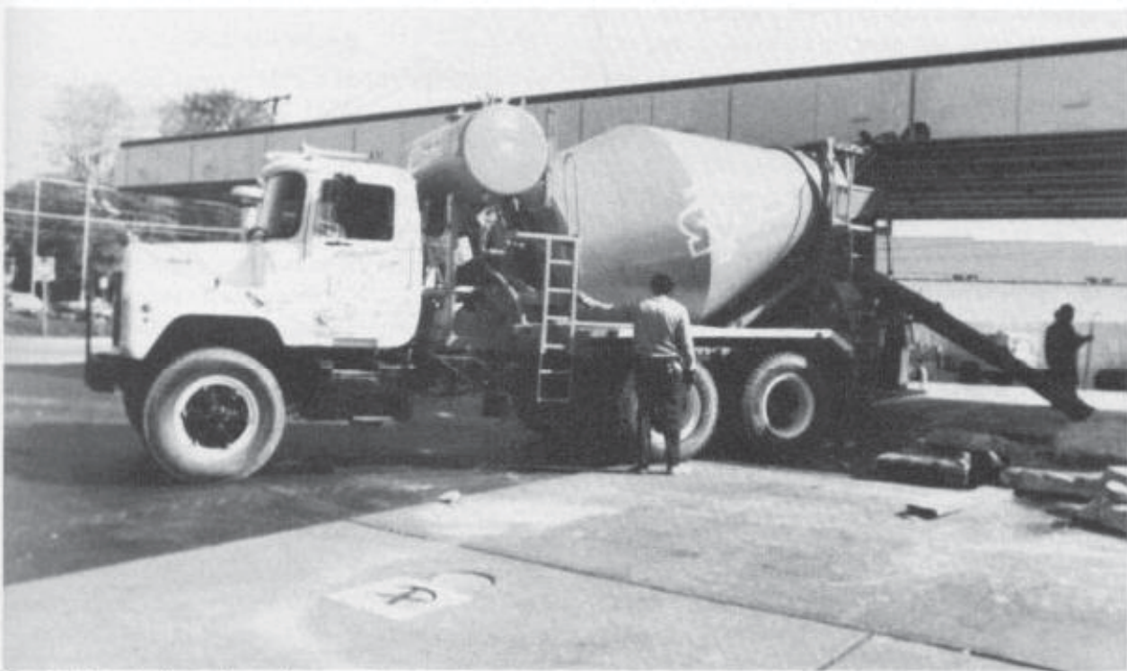
Fig. 4-6. A typical barrel type of concrete truck.
