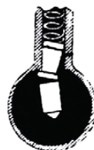
The Side of the mushroom tumbler is hitting the edge of the cylinder
