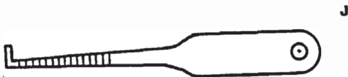
Figure 9C. With a carbide-tip tool engraver, meter your lock pick "J" for picking rotary tumbler locks. Etch lines .050" apart.
