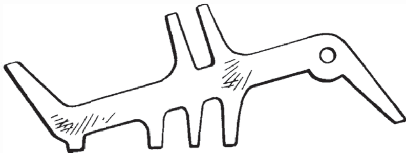
Figure 11. Universal tension wrench called the "Dragon."
