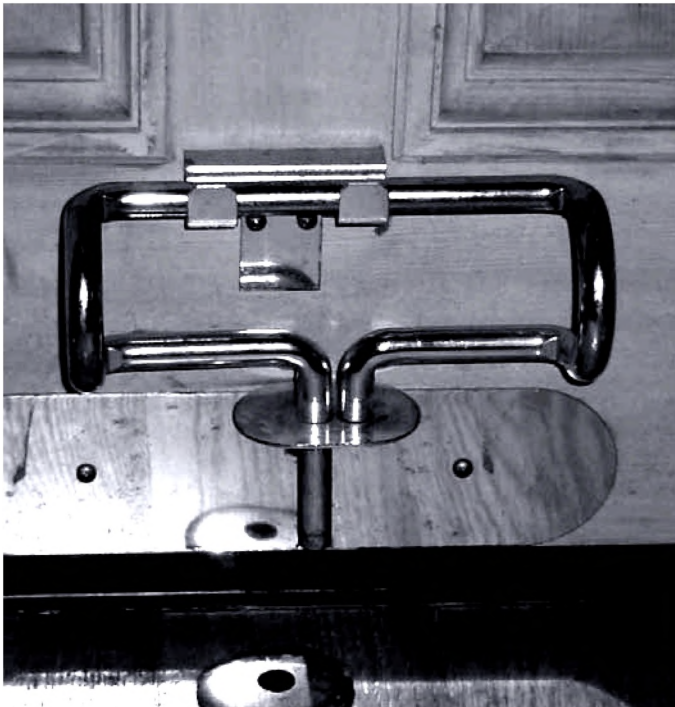
Door block. You can improvise this device with galvanized pipe and sheet metal.
