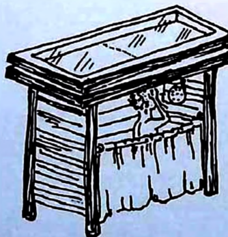
Get free hot water from this simple solar-heated shower.
