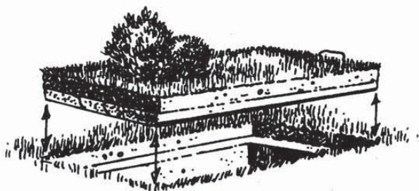
A sheet of suitable material is used to cover the door and turf affixed so that the lid and turf can be removed as one.
