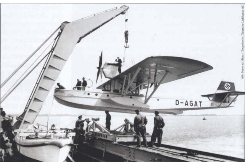
The folding crane lifts the flying boat to the catapult launch system for the next take-off.
