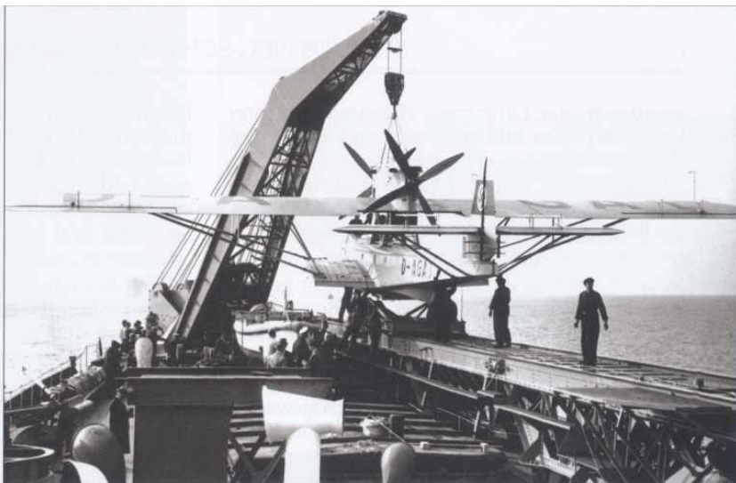
The crane system of the "Schwabenland" must be moved before the flying boat can take off.
