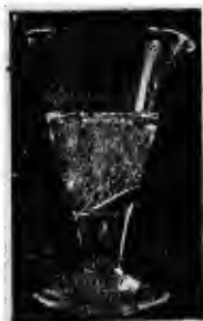
FIG. 56. — Decomposition of water by magnesium containing traces of mercury. (Instantaneous photograph.)
