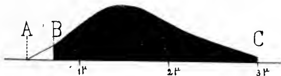
Fig. 15.— Distribution of visible and invisible energy in the light of the electric arc. All the part coloured black represents the energy which, according to Langley, is unused. The part A B is alone used in lighting. The scale here stops at 3 \mu . To make it quite exact, it should be prolonged much farther to the right.
