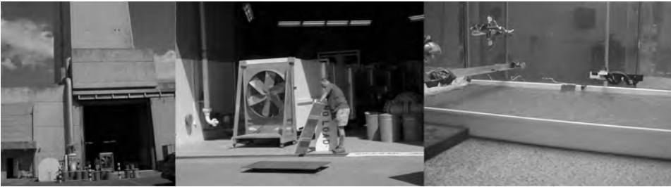
Figure 7.02. A “kitchen sink” experiment in a unique facility. The Mars wind tunnel (MARS-WIT) is housed in a huge airtight building at NASA Ames Research Center ( left ). It contains a small open-circuit wind tunnel ( center ), in which an instrumented tray of water and hydrocarbons ( right ) was installed to study wind-wave generation in extraterrestrial environments.
