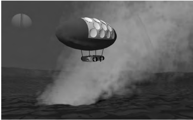
Figure 7.03. A rosy future for Titan exploration? An artist's impression of an autonomous airship exploring a methane vent on Titan. Saturn is visible in the background, and a faint rainbow is cast in the methane steam plume. The disks on the airship envelope form a steerable array antenna to transmit data directly to radio telescopes on Earth. (Mark Robertson-Tessi and Ralph Lorenz)
