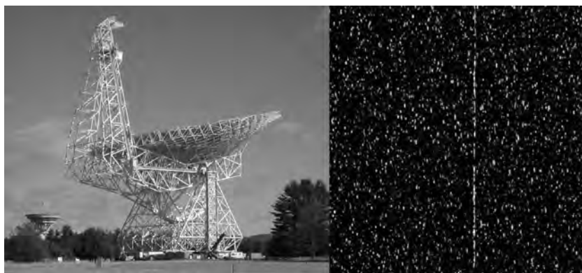
Figure 5.02. Left , the Green Bank Radio Telescope in Virginia, which eavesdropped on the Huygens transmissions to Cassini , and thereby provided the first news that the probe was operating successfully. Right , a dynamic spectrum or “waterfall” chart, like those used by sonar operators aboard submarines. Brightness represents intensity against time (vertical axis) and frequency (horizontal). Random noise appears as spurious dots, but the vertical line denotes a steady signal—that from Huygens . (NRAO)
