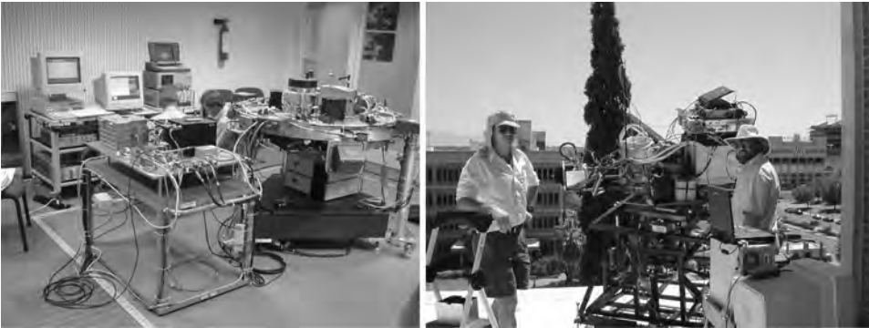
Figure 3.04. The day-to-day business of spacecraft and instrument engineering is not as surgical as figure 3.03 implies. At left is the Huygens probe “engineering model,” the probe equipment deck festooned with wires to verify electrical function. The metal structure is not present. At right is a test of the DISR instrument’s Sun sensor on the roof at the University of Arizona. (ESA and R. Lorenz)
