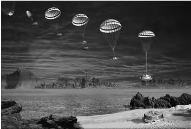
Figure 3.02. A schematic representation of the Huygens descent sequence. After hypersonic entry in its heat shield, a pilot chute pulled off the back cover and allowed the main chute to inflate. This slowed the probe down and allowed the front shield to fall away; thereafter, the main chute was released and the probe descended under a small “stabilizer” parachute. It is pictured here finally operating on the surface. (ESA)
