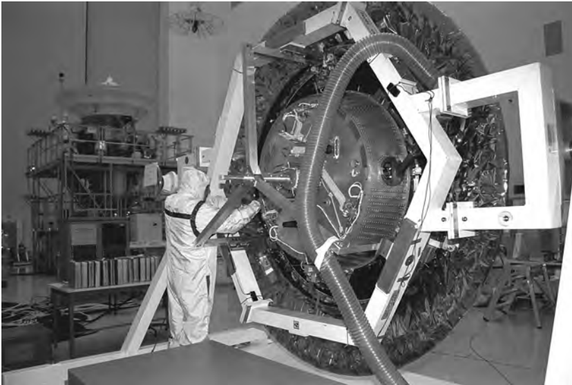
Figure 3.03. An engineer in a white clean-room suit performs some final assembly tasks on the Huygens probe at Cape Canaveral. The front shield is visible behind the white support fixture. Note the cold air hose in the foreground. (NASA/KSC)
