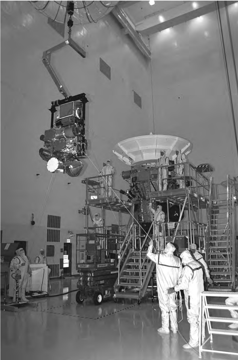
Figure 3.06. Assembly of Cassini at Cape Canaveral. The instrument pallet carrying the cameras and spectrometers, wrapped in gold-colored Kapton insulation, is being lowered toward the Cassini orbiter structure in the scaffold. (NASA/KSC)
