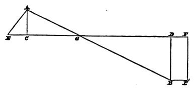
side of the pyramid from base to A. Let  $EF = the \frac{I}{2}$  side of base. Let AB = the length of the floor line of the descending passage-way, intersecting EA at A, and extending to B, or to the foot of DB. Let AC = vertical height of A above EF, the base of the pyramid. And let DB = the vertical height of the base above the point B, or foot of the floor line of the descending passageway. The measures of these various lines, the exactness of which will be shown hereafter, are as follows:
