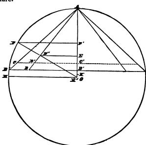
(a.) Let A D B' represent a vertical meridianal section, and A B B' a transverse vertical section (cutting in the corners) of the pyramid. Let D B' =  $\frac{1}{2}$  side of base, and B B' =  $\frac{1}{2}$  diagonal of base. Then,
