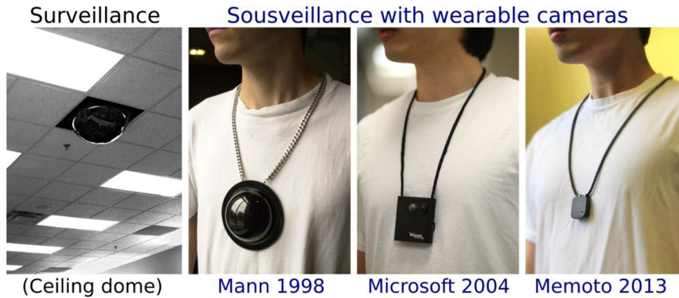
Figure 1. Neckworn lifelogging sensor-cameras. A lifelog is a lifelog (or lifelong weblog) that does not require conscious thought or effort to generate (Mann, 2001).
