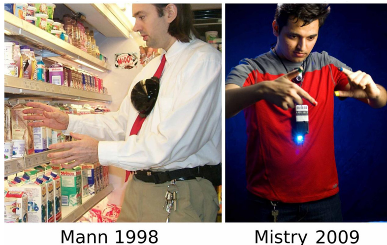
Figure 2. Neckworn Augmented Reality pendant comprised of a wearable camera and projector together on the pendant (Mann, 2001). The wearer can control the apparatus by self-gesturing. Mann referred to the wearable computer in this sense as a “Sixth Sense”, and used the term “Synthetic Synesthesia of the Sixth Sense” (Mann, 2001; Geary, 2003) (Source: Wikimedia Commons).
