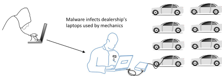
Figure 3.7 It has been suggested that an adversary can attack several vehicles by targeting the laptops of mechanics at a dealership.
