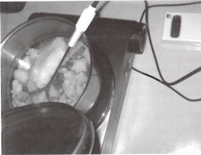
A small amount of material might be heated to its melting point to check quality. In this case the melting point was verified during the mix.
