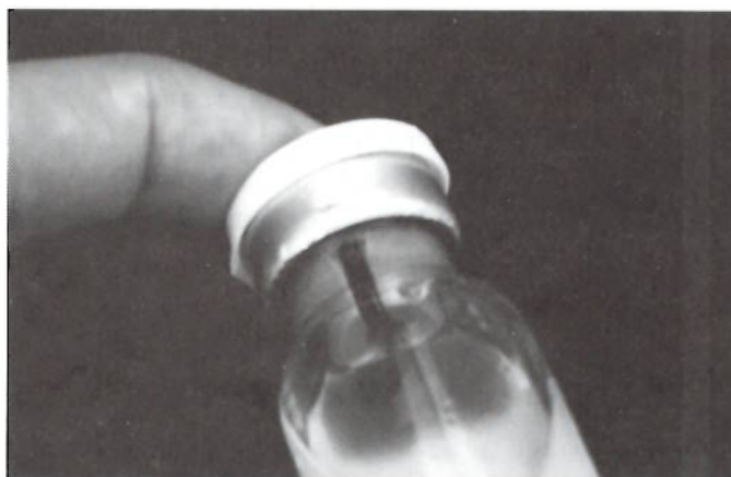
This crimping on this product is poor, which may lend itself open to contamination from the outside air.
