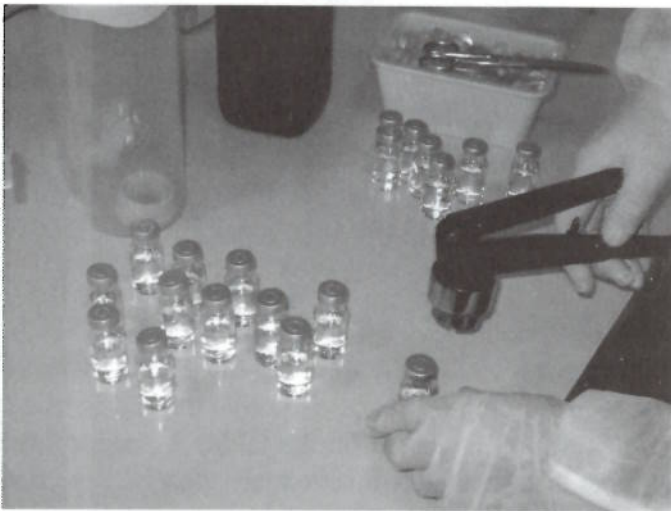
The vials are sealed with the use of a hand-crimping device. Vials and rubber stoppers were sterilized in ethyl alcohol before filling.
