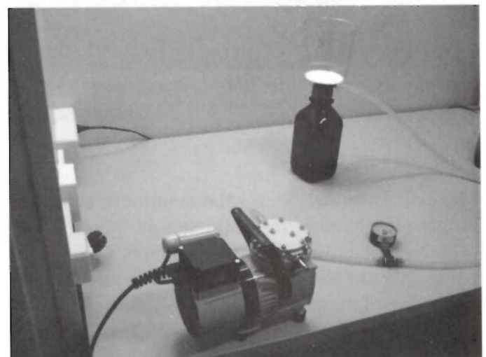
The disposable Nalgene filter is screwed onto the top of a 1 liter bottle. The vacuum suction hose is attached.
