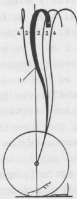
Figure 9. Zones of the barbell's movement: 1- optimal; 2- less advantageous; 3- fixation with great difficulty; 4- a miss or a success by chance
