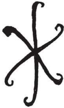
The "German man" as masonry anchor
