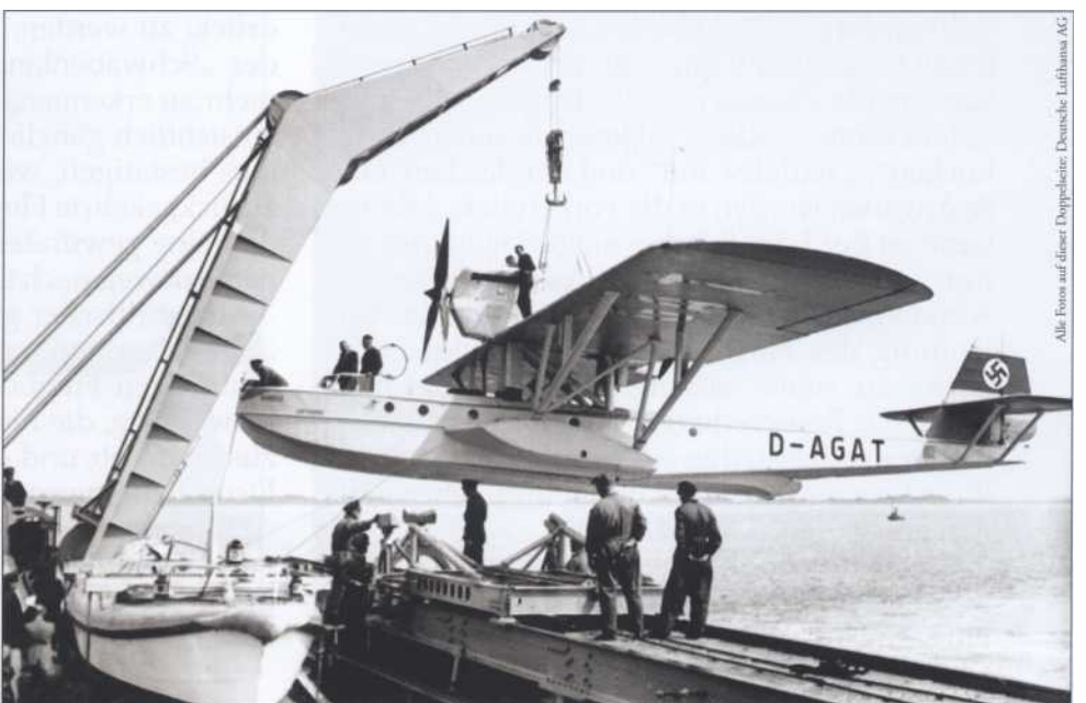
The folding crane lifts the flying boat to the catapult launch system for the next take-off.
