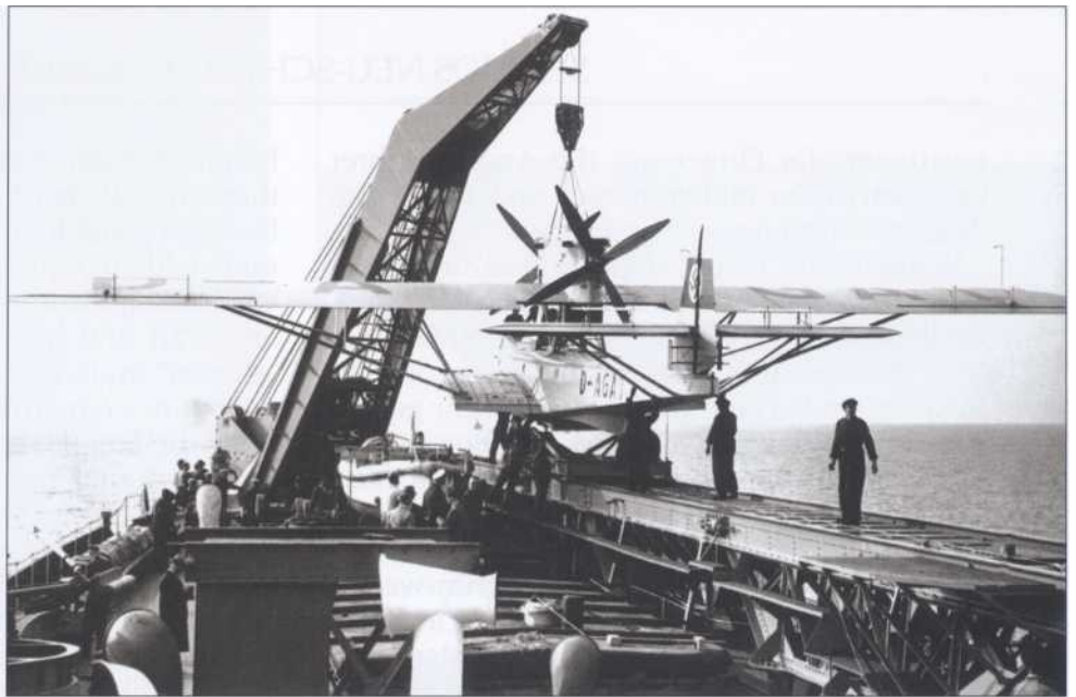
The crane system of the "Schwabenland" must be moved before the flying boat can take off.
